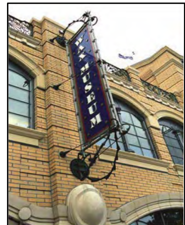
Figure 7.11 Vertical projecting sign.
