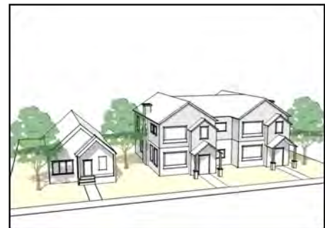
Figure 5.13 Multi-family unit with front facade step-back
