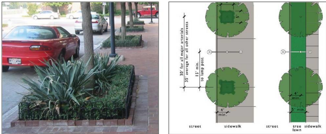
Figure 5.46 Ornamental tree guard and raised tree curb (left), and tree well and tree lawn landscaping (right).
